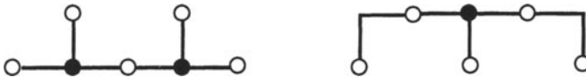
Figure 2.16 A 5-point example where the IIS performance ratio is \frac{7}{6} . The optimal SMT (left) has cost 6, while the (possible) heuristic output (right) has cost 7.
