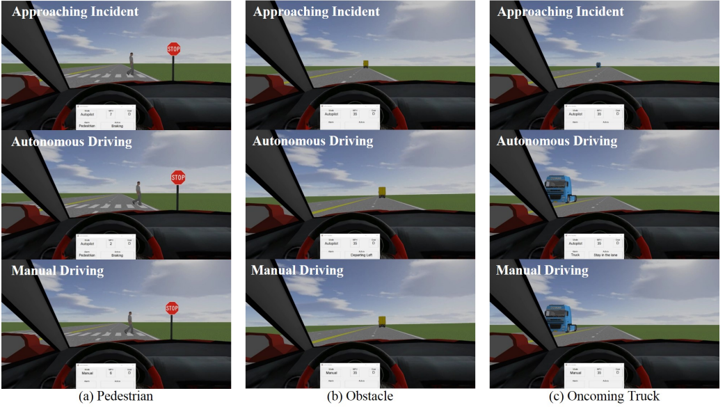
Fig. 4. Screenshots of driving videos used in the online user study, covering three types of incidents: (a) a pedestrian crossing the road, (b) an obstacle (a stopped truck) ahead of the lane, (c) an oncoming truck in the neighboring lane. Each sub-figure shows: (top) the driver’s view when the automated vehicle is approaching the incident, (middle) the view of autonomous driving if the driver chooses not to take over, (bottom) the view of manual driving if the driver chooses to take over.
