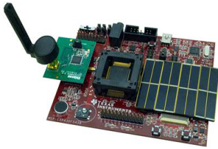
Fig. 1. Energy harvesting wireless sensor node that uses an MSP430 and solar energy harvester module based on the bq25504.
