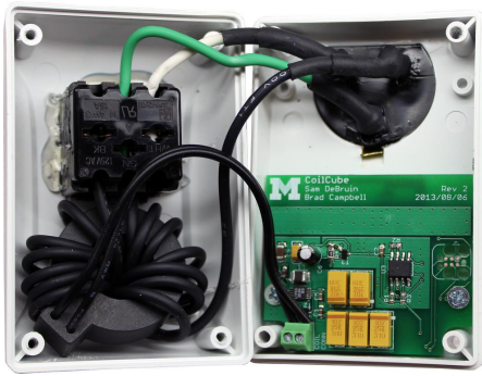
Figure 19: Monjolo sensor in plug-load form. The case is open so that the female socket is visible on the left and the male plug is visible on the right. The energy-harvesting power supply is visible in the lower right PCB. The Epic Core is attached to the opposite side of the same PCB.
