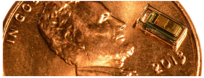
Figure 12: A mm-scale sensor node that integrates a solar cell, processor, radio, and battery that provides much of the pulse sensor functionality. This illustrates that the “peel-and-stick” sensor tags we envision will soon be viable.
