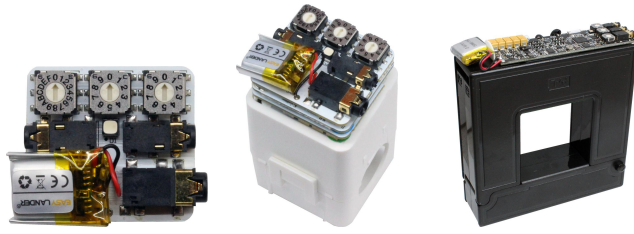
(a) Config Board (b) Expanded Meter (c) High Current Meter Fig. 5: Triumvi configuration board and high current version.
