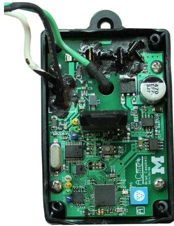
(a) Voltage Monitor
