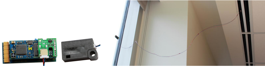
Figure 7.4: Breeze airflow sensor. The solar energy harvester is placed near a light source, such as a window, and a MEMS airflow sensor is placed near an air vent. When the harvester has sufficient energy it samples the airflow sensor and reports its readings. Decoupling the harvesting from the measurement point enables both faster sampling and a smaller sensor.
