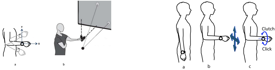
Figure 1. Left: Pointer manipulation in the rotation techniques, W1RR and P1RR, is governed by the orientation changes of the control device. (a) For W1RR, the user must sweep the entire forearm to cause changes orientation of the smartwatch. (b) For P1RR, the user can use the wrist sweeps as a more subtle form of manipulation; Right: W1RR can calibrate the center frame of reference from inactive state (a) to raising the arm in front (b) to switch to manipulation mode. From this mode, a 45° wrist flick outwards and back can be used to trigger a click action (c).
