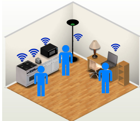
(c) Multiple users in the room receives broadcast from appliance motion tags, however, motion matching ensure correct detection of user-appliance interactions
