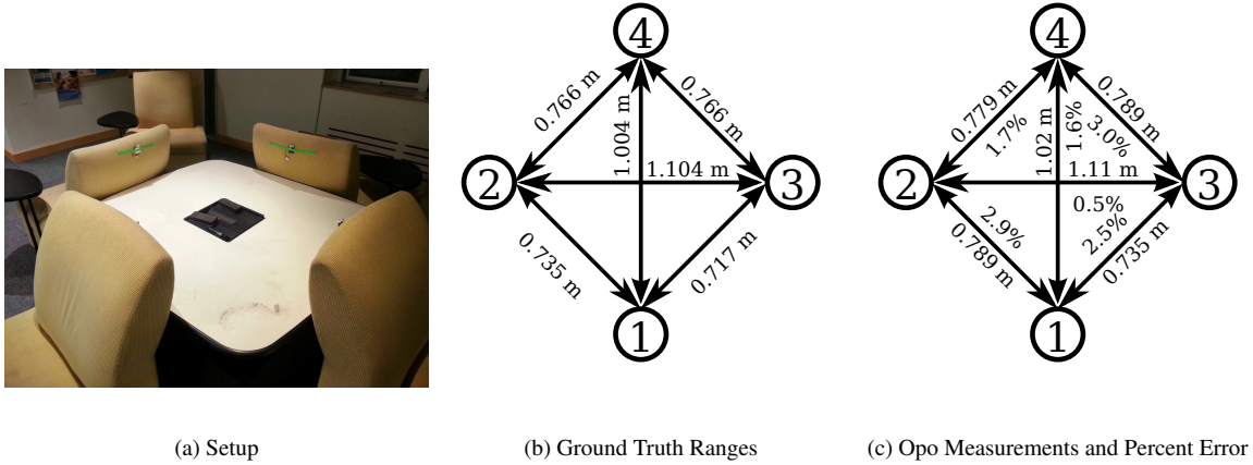
Figure 6: Four-Way Ranging Accuracy: Setup (6a), ground truth (6b), and Opo measurements (6c). The measurements shown in 6c are the median measurements between each pair of sensors, aggregated over the duration of the experiment (12 min).
