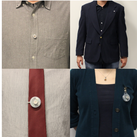
(b) Various different wearing scenarios of Opo. The Opo in the upper left is a shirt button; the Opo in the upper right is a lapel pin; the Opo in the bottom left attaches to a tie clip; the Opo in bottom right is a badge clip.
