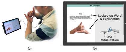
Figure 17: The ASL Dictionary application: (a) a deaf person looking up an ASL word “help”; (b) a screenshot of the tablet application.
