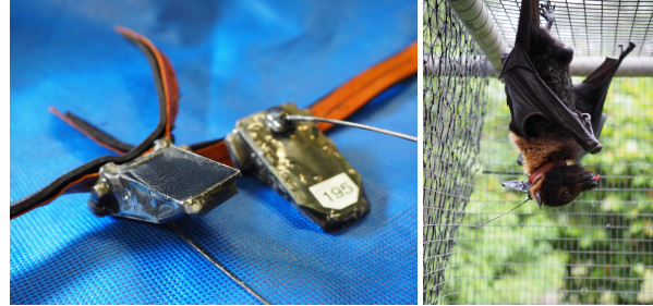
Figure 5: Camazotz collars (left) and a spectacled flying fox ( Pteropus conspicillatus ) with collar (right).
