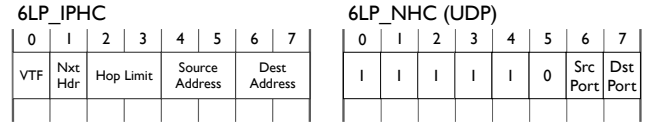
Figure 3: Header Compression Format. The encoding formats specify what fields are carried inline.
