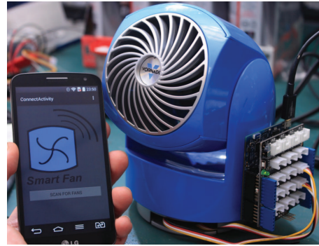
Fig. 6: 802.15.4 and BLE connected prototype smart appliance
