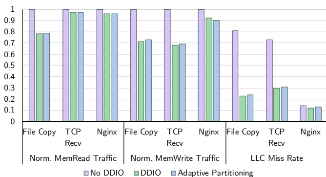
Fig. 15: Memory Traffic and LLC miss rate of our adaptive partitioning defense vs. DDIO.
