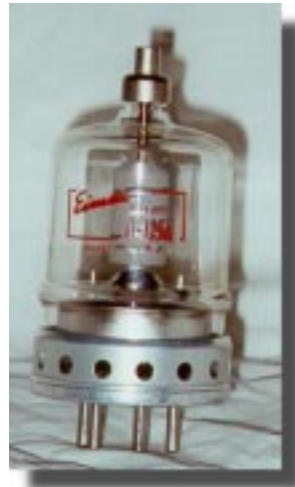
Power triode: similar in size to power tubes used on the early computers, but this particular tube type is brand-new. It can be compared with a power transistor of comparable power rating.
