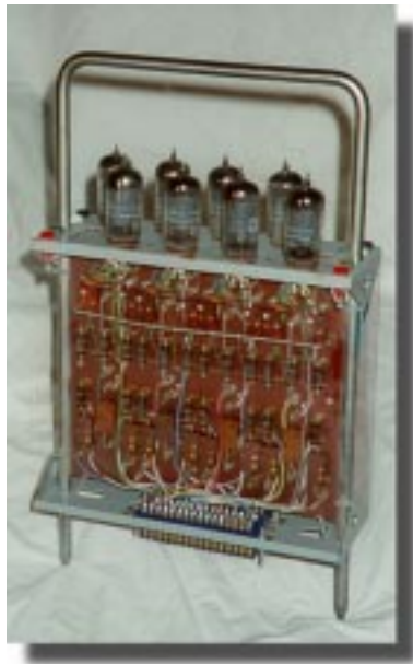
A single digit from the accumulator of a Burroughs 205, circa 1954. The 205 was a decimal machine with a magnetic drum for primary memory. This device, about the size of a modern laptop, stored one decimal digit (i.e., 4 bits!)
