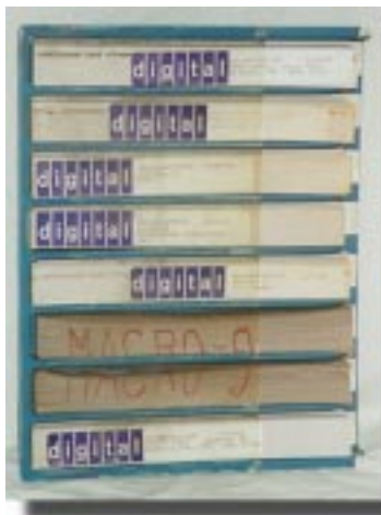
A "DEC tape" - a magnetic tape used on several early DEC computers. It was notable in that it was addressable: one could move forward or backward to a specified tape block. This particular tape contains the source code for the first Pascal Compiler, written by the inventor of Pascal, Nicklaus Wirth.
