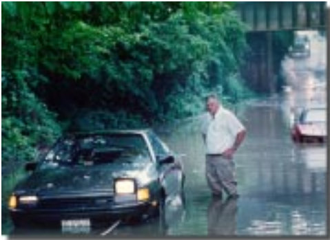
Emeritus Professor Alan Batson discovers the hard way that water is an incompressible fluid: while driving through a large puddle, his engine sucked in rainwater through the air intake and literally blew apart on the compression cycle (the headlights then kept blinking on and off - an interesting failure mode of the electrical system)
