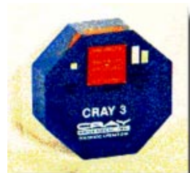
A gift from Cray Computer Inc., containing three GaAs chips that were to be part of the Cray 3 computer. The large brownish item in the center is a miniature "printed circuit board" — the idea was to bind the chips directly to this board (rather than to first package them in individual carriers) — this allowed smaller, denser packaging.
