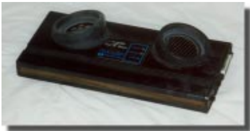
Acoustic coupler - a 10 characters/second "modem". In use, the telephone handset was placed in the rubber cups. Communication was established through audio tones with no electrical connection between computer and telephone line. Such connections were generally limited to <300 bits per second and were often favored since prior approval of the carrier was (assumed) not necessary.
