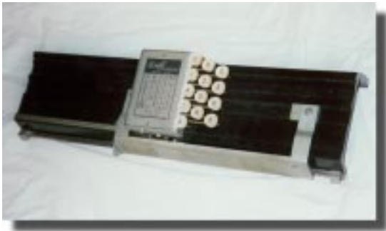
Manual card punch from Wright Line. Numeric digits could be inserted directly from the keys. Alphabetic and special characters required 2 or 3 holes obtained by pressing all needed keys while holding down the 'S' key at bottom until finished. This was the "laptop" version of a keypunch machine!
